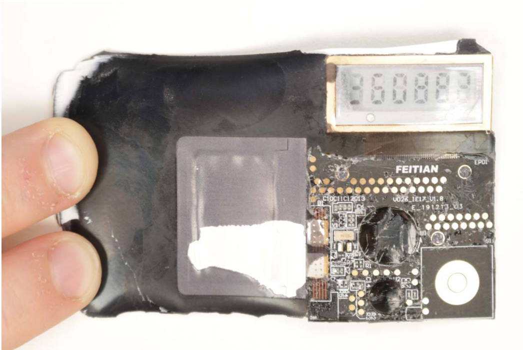
Figure 31: PCB front side after scratching away a protective coating
