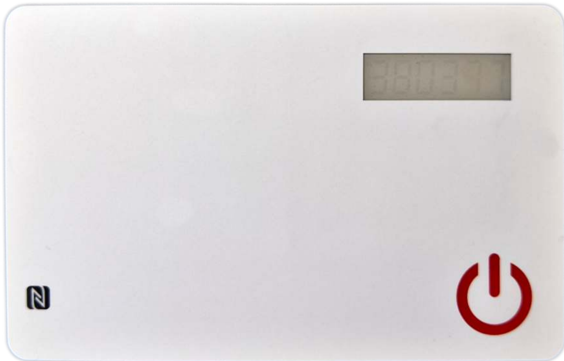
Figure 17: Deactivated OTPC-P2 token with the last OTP still slightly visible
