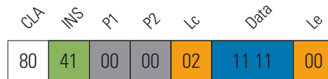
Figure 15: Modified data in “get time and serial number” command returning the current time twice
