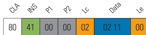
Figure 4: Example: APDU to query the time and serial number of the card
