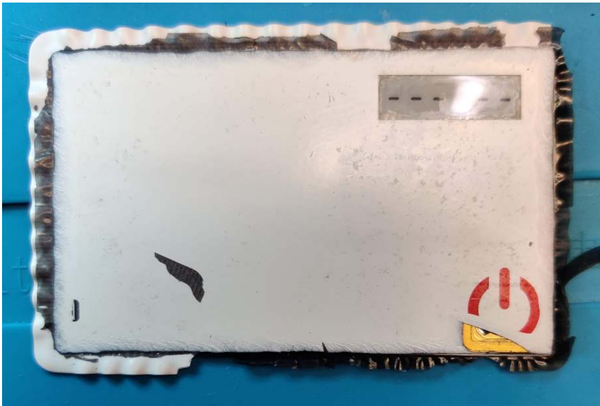
Figure 5: Card is only slightly damaged/dissolved by acetone (image by Philippe Teuwen)
