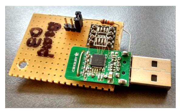
Figure 7: SPI read and write access to a Cherry USB dongle (thanks to Alexander Straßheim)
